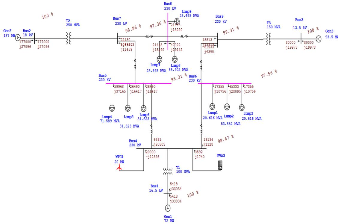
FIGURE.9. Power flow analysis for the system with PV and wind
