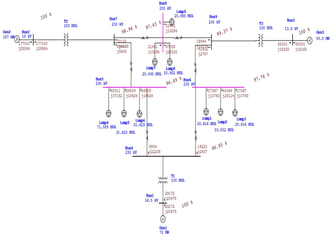
FIGURE.2. Power flow analysis for the normal system
