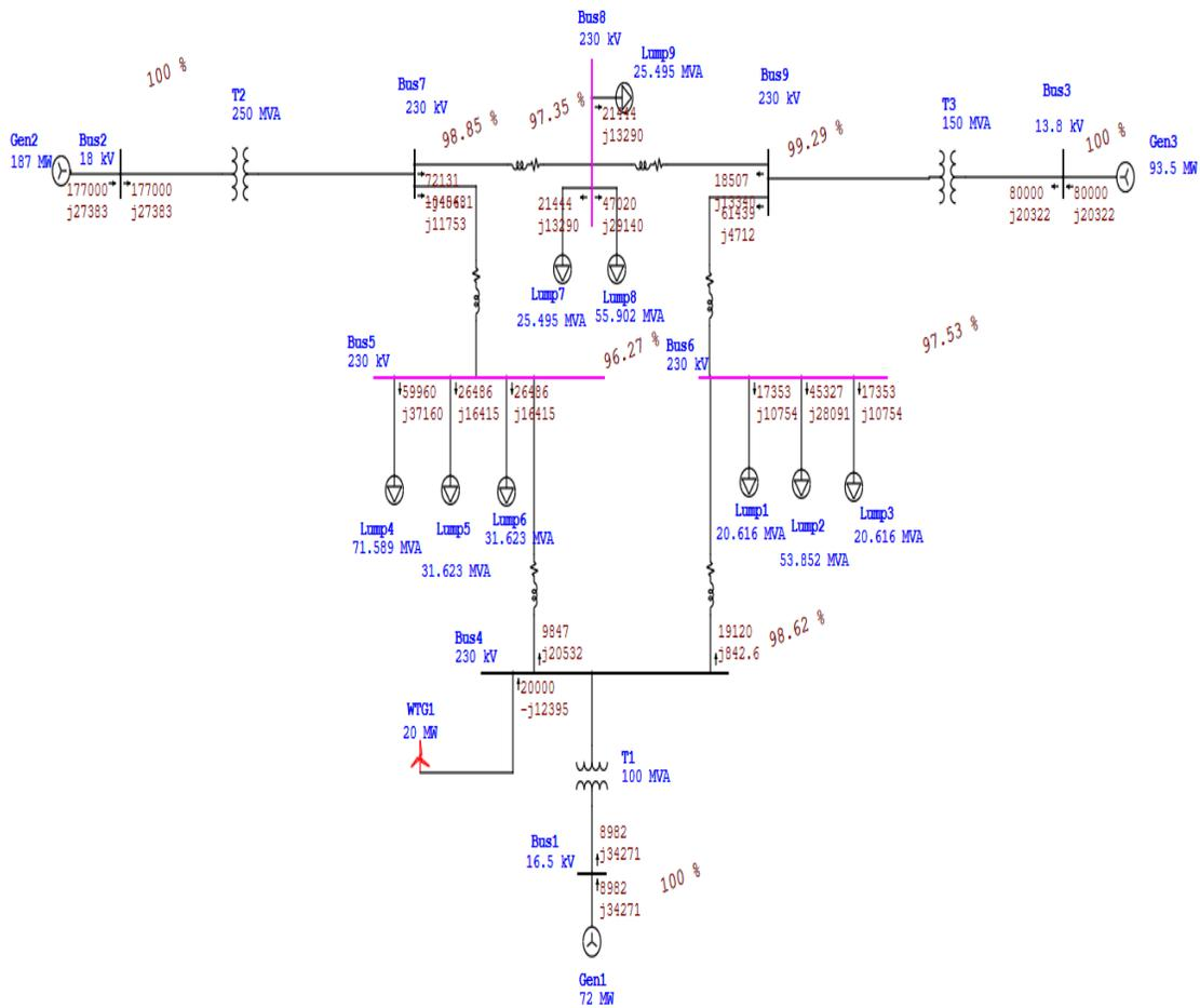
FIGURE.6. Power flow analysis for the system with wind turbine
